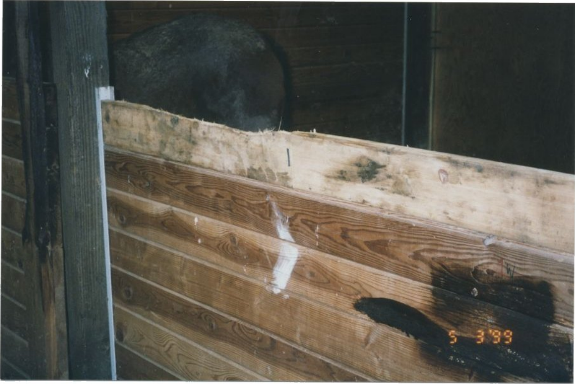
Figure 1. Top board in one of the ten stalls used in this experiment. The left end of the board is Douglas Fir while the right end is Western Juniper. Note the amount chewed from the Fir portion of the board compared to the Juniper.
