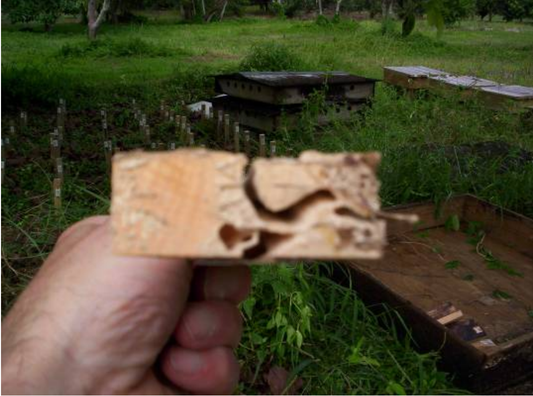
Figure 3. Example of termite attack on the sapwood portion of a mixed heart/sap western redcedar sample exposed to formosan termite attack for 6 months in Hilo, Hawaii.
