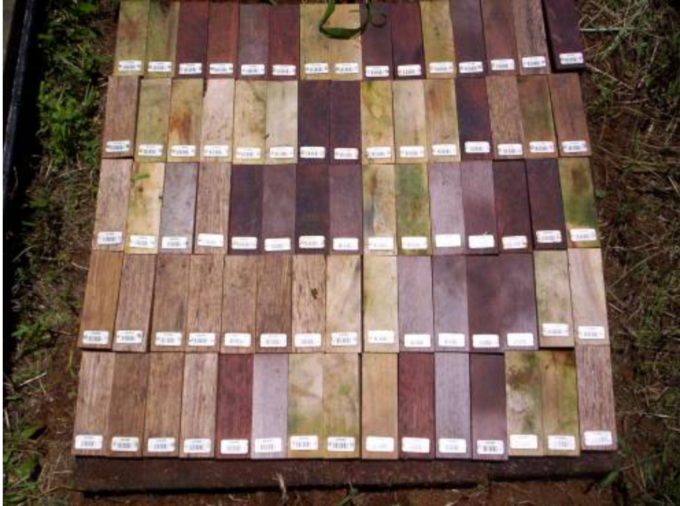
Figure 2. Reassembled ground proximity decay test after 6 months of exposure. Materials in this array include two naturally durable tropical hardwoods, merbau and ipe.
