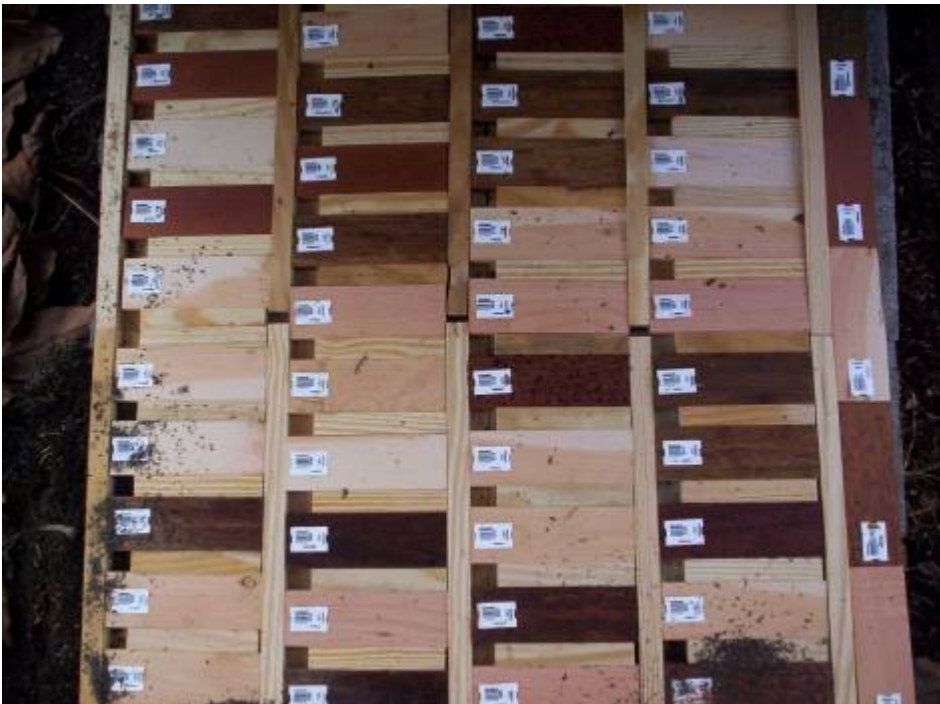
Figure 1. Example of test samples in a termite array one month after installation..
