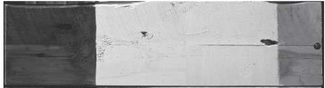
Figure 1. — Saw-textured and smooth-planed surfaces of vertically exposed lumber at test site near Madison, Wisconsin.
