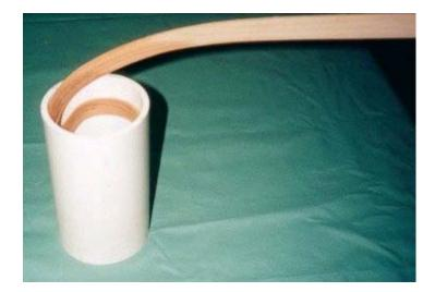
3 inch-diameter PVC pipe with partially-inserted 1inch wide heated, water-soaked strip. A strip this long will generally have to be reinserted into the boiling water tank 2 or 3 times before the strip is completely loaded into the form.
